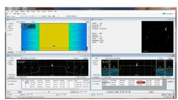
Fast validation of LTE base station transmitter with push button preset, and pass/fail
