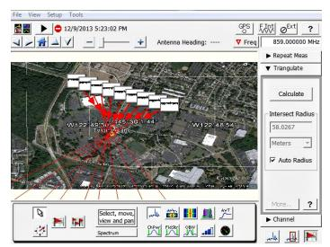
Locate interference with integrated mapping solution and triangulate multiple measurements with resulting areas of uncertainty
