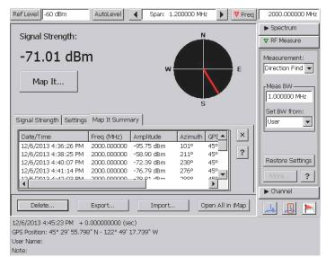
Use Direction Finding display - use compatible antennas and field strength measurements to find the likely directions to signals of interest. Results can be sent to the Mapping application for further geolocation analysis.
